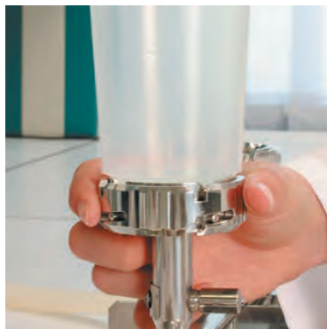
2. Membrane is placed onto the filter base and the funnel installed
