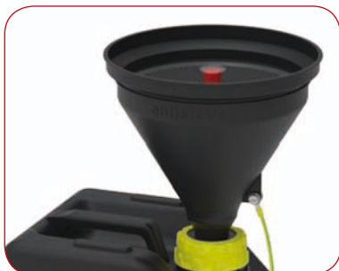
b.safe Funnels 180 with Level Indicator (Cat. No. R 840-16). Optic Level Indicator that is permanently mounted in the funnel. As soon as the red pin fills the inspection glass completely, the canister is full and has to be exchanged.
