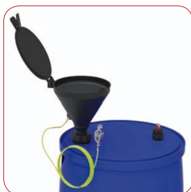
b.safe Level Indicator for Barrels (Cat. No. M 730-01) for the assembly on female threads G3/4". Liquid waste is filled into a barrel via a b.safe Funnel 180 (Cat. No. R 880-10) for barrel thread G2". At the same time, you can keep an eye on the fill level through the integrated optic Level Indicator during filling.
